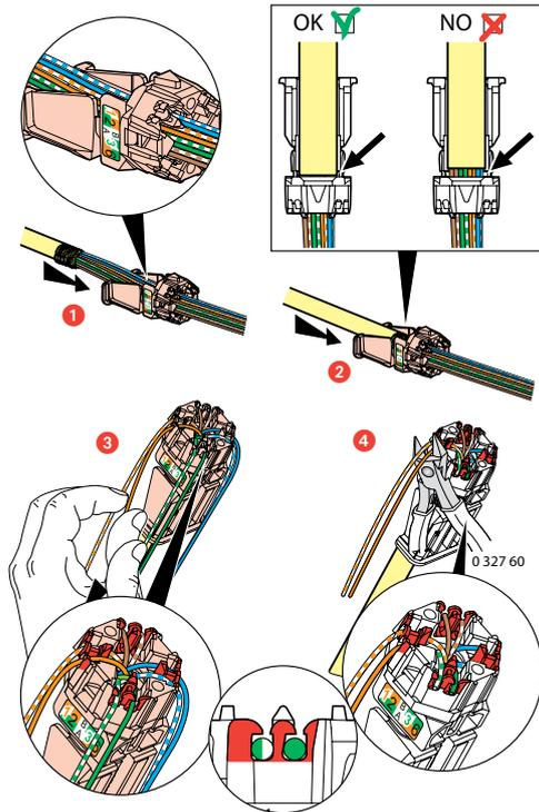
Spreading the cables and positioning the sleeve firmly in the spreader ensures that a pair-breakage distance of 13 mm is kept between pairs, as required by the standard.
