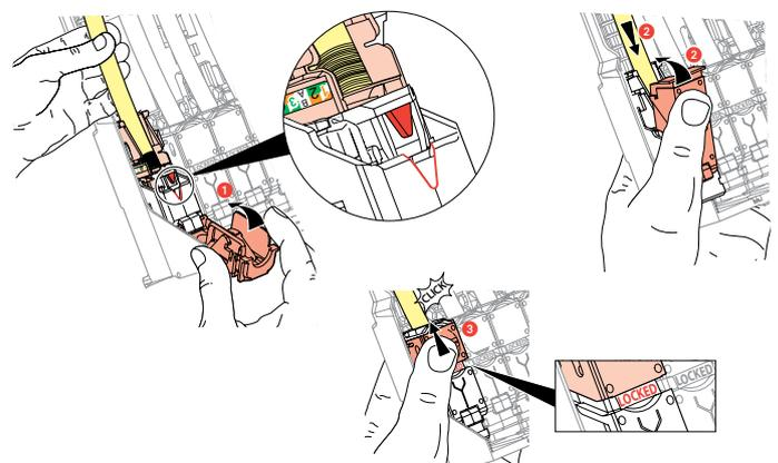
This system makes it easy to spread pairs before fitting them onto the connector.
